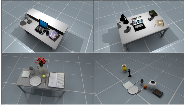
Figure 6. Example of a generated scene layout for robot learning environments, illustrating the placement of interactive objects and background assets to ensure a collision-free, physically plausible layout.
