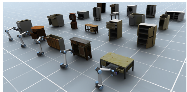
Figure 5. Articulated 3D objects generated by predicting a part-decomposed structure, synthesizing part geometry and appearance, and estimating articulation parameters for physics-based simulation (Liu et al., 2026).
